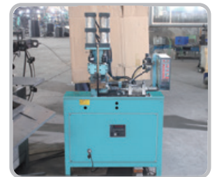
⑪ Butt welding machine
