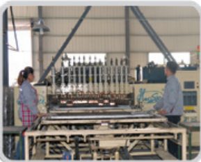
⑤ Gantry welding
